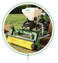
Surface reseeding with the **Seeder Kit**. The seeds are evenly blown between the tines. The **Roller Kit** then compacts the surface.
