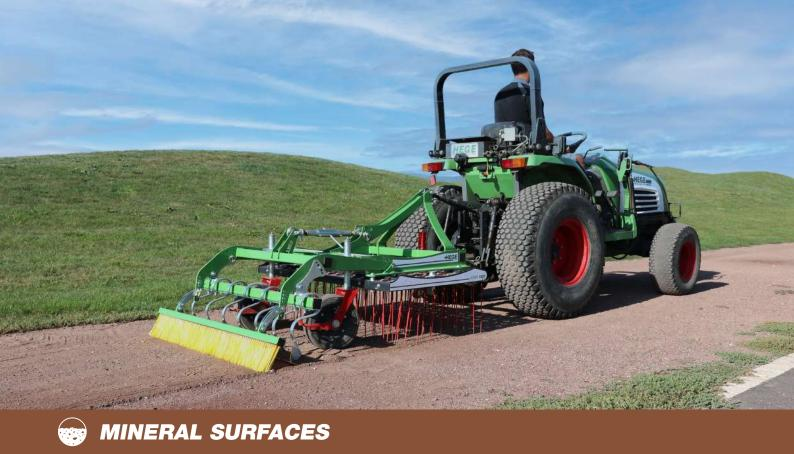
Designed for pesticide-free maintenance of fine-grained surfaces: shale, limestone, pozzolana, ash...
