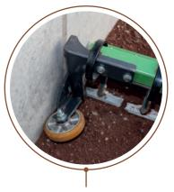
Weed right up to the edges without damaging the blades or the edge, using the **Edge Kit**.
