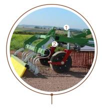
1- The blade working depth can be set using the 3-point push bar.
