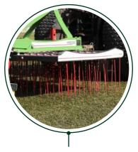
High tine density (tine spacing of 4.6 mm, 0.18"): exceptional output up to 20,000 m²/h (215,278 ft²/h).
