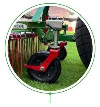
The **Front Wheel Kit** perfectly follows the ground contours to ensure even grooming over the entire surface.
